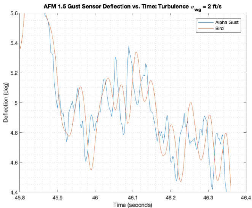
Figure 4.9 von Karman Turbulence Gust Sensor Response
